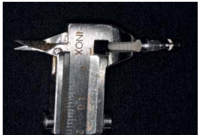
Fig. 2 Marking the defined implant surface with calipers
