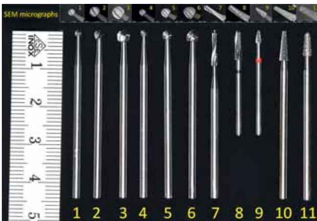
Fig. 1 Overview and SEM micrographs of the investigated rotating carbide burs (Nos. 1–10) and the reference shoe (No. 11)
