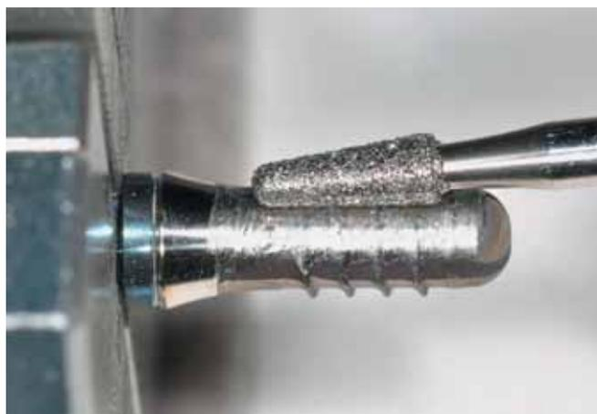
Fig.3 Processing of an implant with the reference abrasive No. 11
