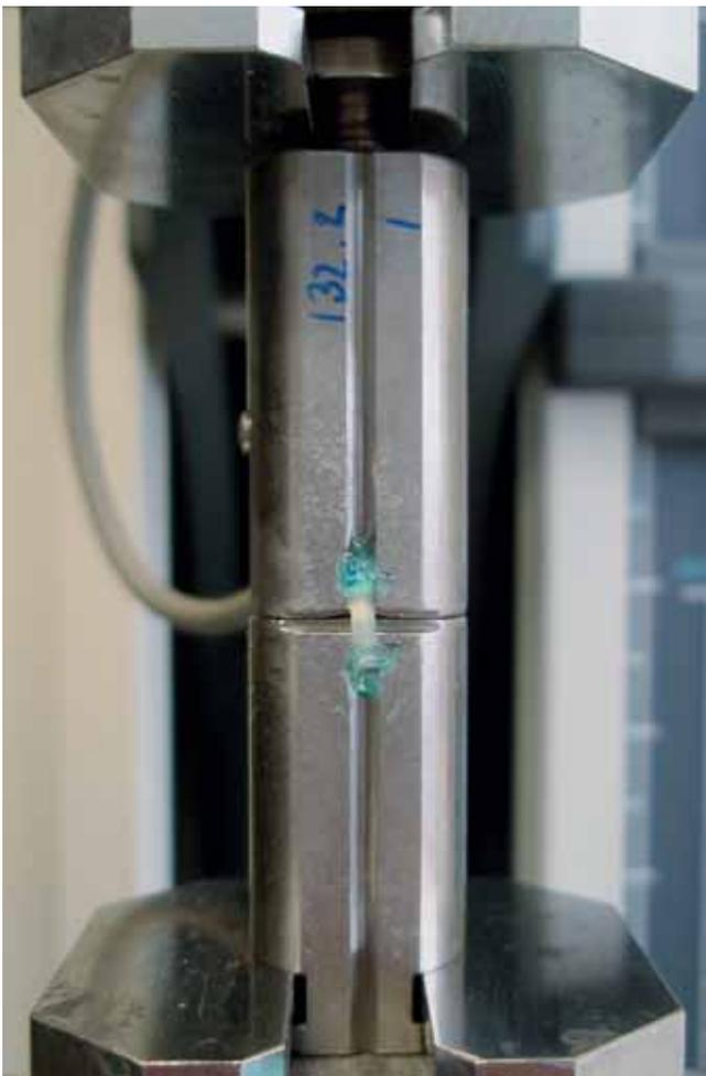
Fig.2 Microtensile test, in which the dentin/composite stick is attached to the jig with superglue.
