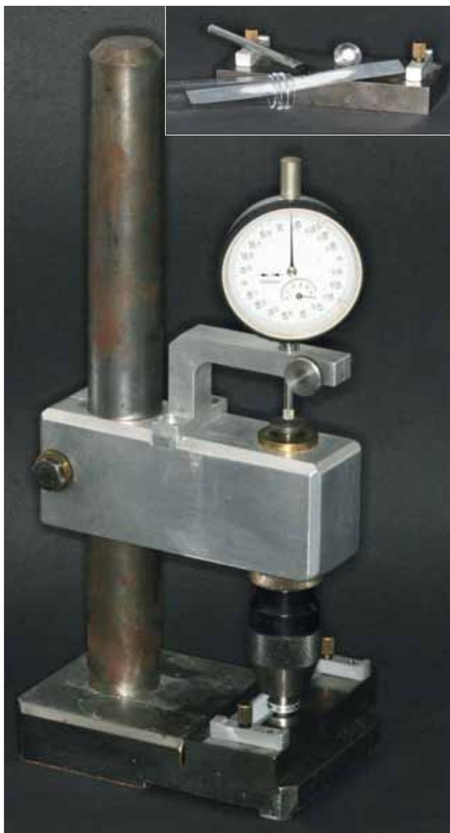
Fig. 1 Large image: custom made apparatus for controlled dental hard substance abrasion testing. Small image: Abrasion slide with a sample attached in the holder as well as a sandpaper strip with abraded enamel powder.
