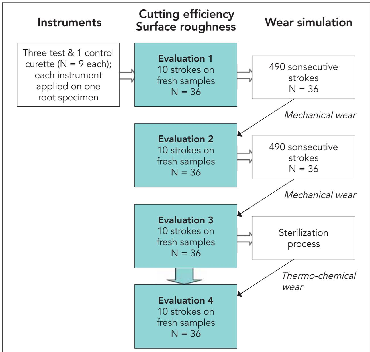
**Fig. 3** Flow-chart of the experimental set-up. Nine instruments per test group were evaluated for dentin removal, without sharpening, at defined points. At the initial and before three following 10-stroke dentin collection points, fresh dentin samples were used to insure standardized surface characteristics at the test phase.
