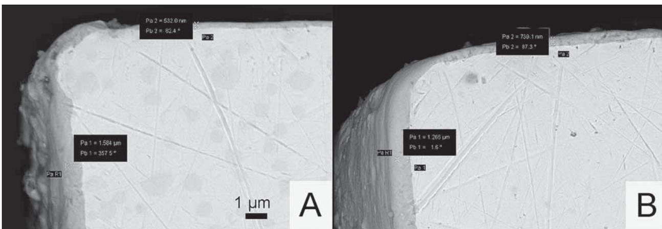
Fig. 2 Detail SEM images of the coated currettes (A: Dep-S, B: AmE) at a magnification of 10,000×. The thickness of the coating varied between 0.4 and 1.7 µm for the Dep-S and 0.6 and 1.4 µm for the AmE.
