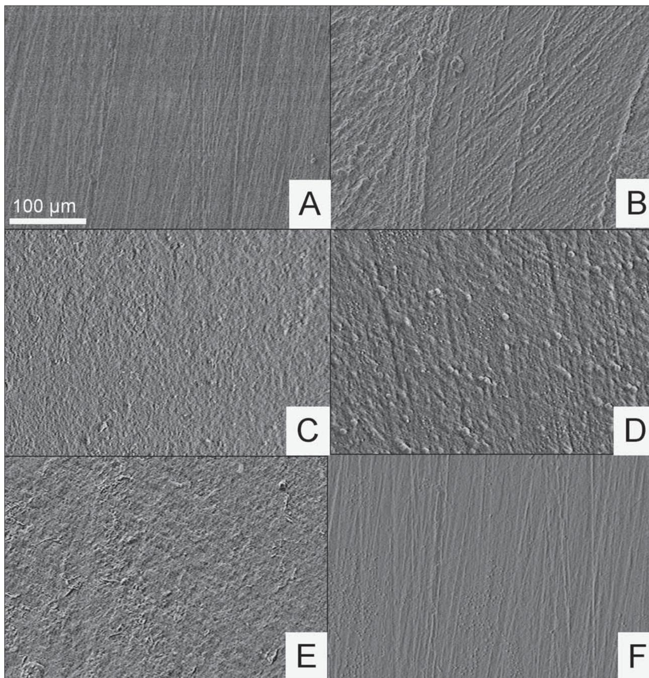
**Fig. 4** Panel A represents a polished dentin surface before curette treatment. Panels B–E show representative SEM images of dentin surfaces after ten strokes on polished dentin samples, after total wear of 1,010 strokes (B: Dep-N, C: Dep-S, D: AmE, E: HuF). Panel F shows a representative dentin surface treated with the AmE instrument after the sterilization process. Note the resemblance to the polished dentin surface at baseline.
