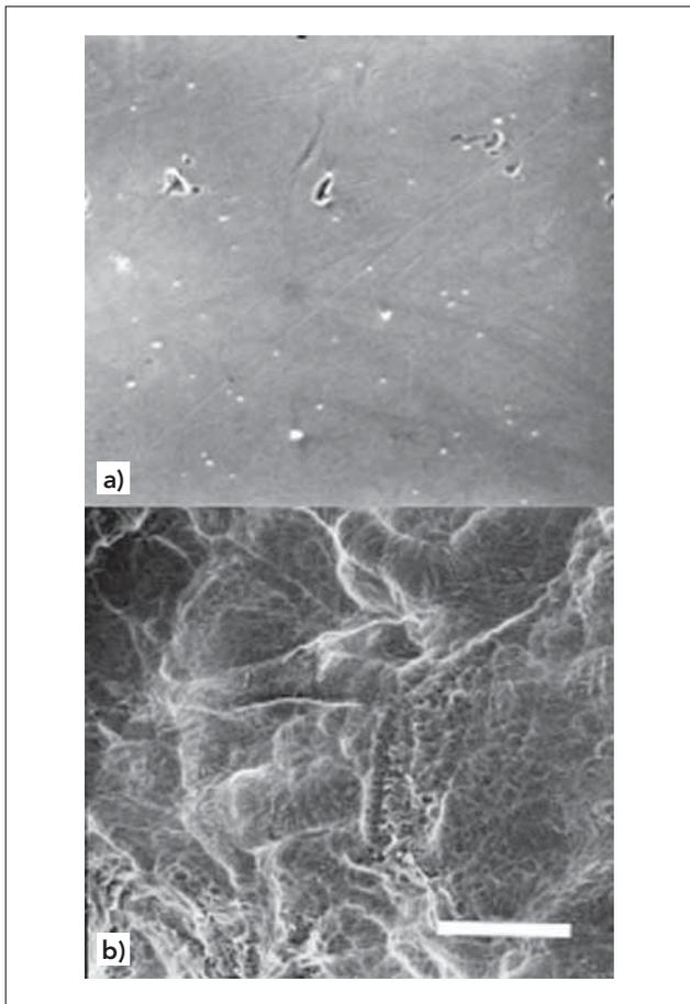
Fig 1 Surface architecture of pure titanium discs. Scanning electron micrographs of a) machine surfaced (MS) and b) sandblasted/acid etched (SE) surfaces. Scalebar = 50 micrometers.
