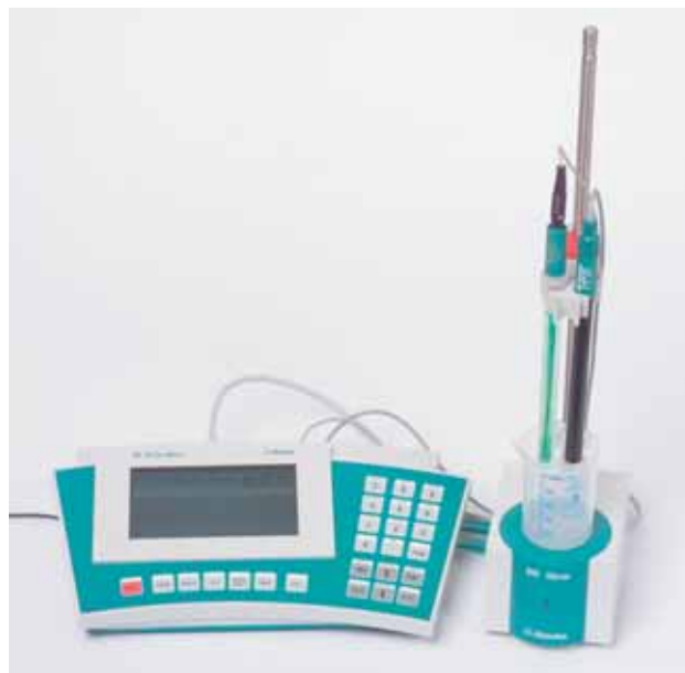
Fig. 1 Measuring equipment for direct potentiometric determination of the fluoride content in food grade salt (Mettler, Herisau)
