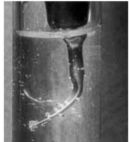
Kavitation am EMS-Instrument
