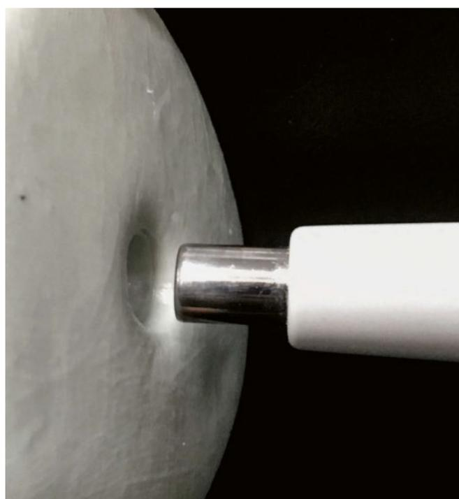
Fig.2 The silicon guide used for accommodating the tip of the spectrophotometer during color evaluation.
