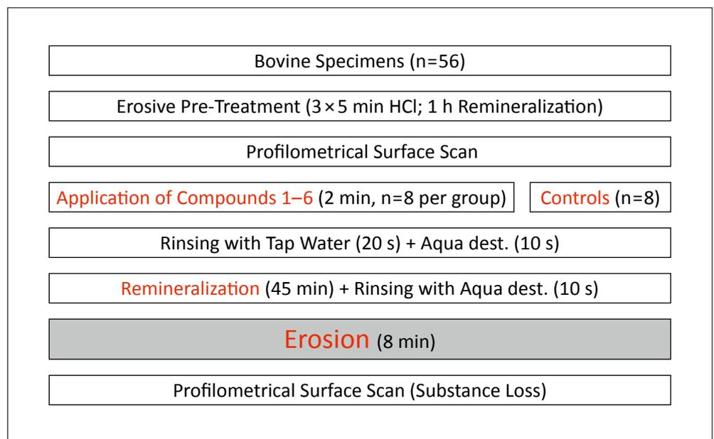
**Fig. 2** Set-up of experiment 2, with eight erosive/remineralizing cycles
